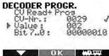
Some CVs are made up of so-called binary values. This means that multiple settings are combined in a single value. Each function has a bit location and a value. If such a CV is to be programmed, all values must be added. A disabled function always has a value of 0 and active function will have the value indicated in the table. Add all active values and program the result into the CV. The Navigator automatically shows the bit conditions in the lowest row of the display for control.
