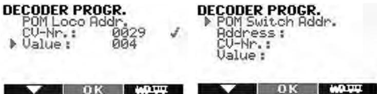
The PoM programming method is the only process to directly program operations on the rail track. All CVs in the decoder except CV 1 can be programmed using the PoM programming method.
