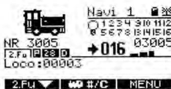
If the locomotive address has been correctly selected, the data associated with the locomotive will be shown in the display. Those data include: locomotive address, locomotive name (if assigned), light, functions 1 through 8 and of course the direction of travel and the speed step.
