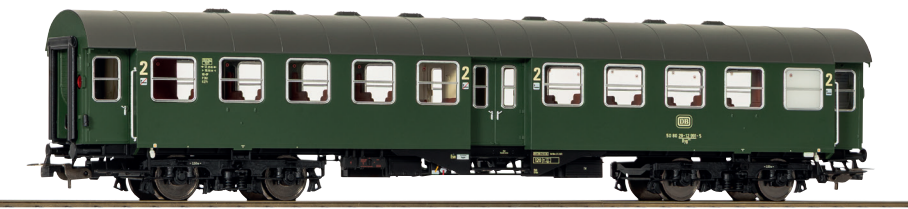
58863 2nd class Conversion car B4yg DB IV, with Minden-Deutz bogies MD41
