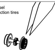
If used frequently, oil the wheelsets with a drop of non-resinous, acid-free sewing machine oil! In order to achieve the best possible running and traction properties, it is advisable to run the locomotive in for 25 minutes forwards and 25 minutes in reverse without load. Clean rails are essential for good performance.
