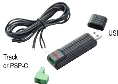
Connect a track or the PIKO SmartProgrammer-Connector (PSP-C) to the track connection of the PIKO SmartProgrammer-Stick using the green plug. Now plug the PIKO SmartProgrammer-Stick into the USB port of your device. The control LED on the stick will flash several times.
