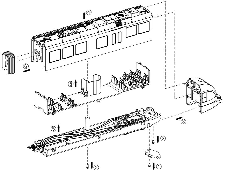
Antriebscontainer Elektro / Powered Container electric / Contenant Drive
