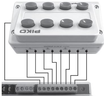
The programming in analogue mode is similar to digital programming. Besides the two servo control buttons ("address") there are two more buttons necessary to act as [+] and [-].
