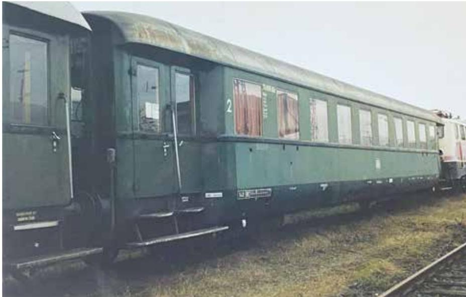
At the beginning of the 1930s, the DRG began building four-axle express train coaches to replace the older state railway designs with their three-axle running gear with more comfortable designs. Thus, over a period of about 15 years, various types of express train coaches were developed, culminating in the coaches of the type 42.
