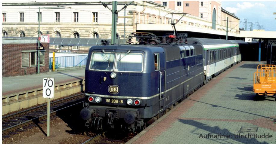
In 1972, the Deutsche Bundesbahn ordered dual-frequency locomotives under the designation 181.2 for traffic to France and Luxembourg. According to its The 25 locomotives were delivered on cross-border routes at speeds of up to 160 km/h in express service, including in front of the famous Orient-Express.
