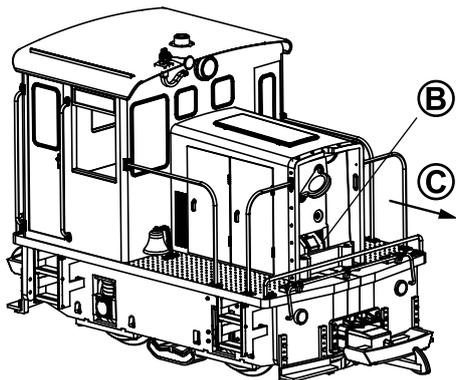
**A** Pull top of radiator panel forwards, then pull panel upwards to remove it.
