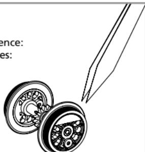
If used frequently, oil the wheelsets with a drop of non-resinous, acid-free sewing machine oil! In order to achieve the best possible running and traction properties, it is advisable to run the locomotive in forward 25 minutes and reverse 25 minutes without load. Clean rails are essential for good performance.
