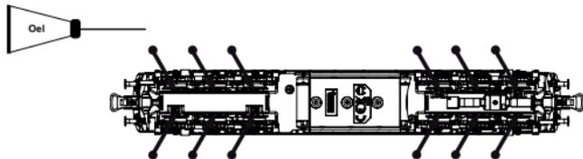
If used frequently, oil the wheelsets with a drop of non-resinous, acid-free sewing machine oil! In order to achieve the best possible running and traction properties, it is advisable to run the locomotive in for 25 minutes forwards and 25 minutes in reverse without load. Clean rails are essential for good performance.
