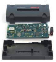
Attention! To avoid any possibility of short circuits cover the screw heads with electrical tape.
