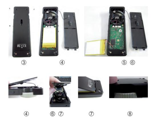
\*In case the wire attached to the cover is accidentally removed from the main circuit board. It can be easily plugged into the main circuit board again. The plug can be inserted either direction. For easier assembly we suggest placing the wire towards the front of the unit.
