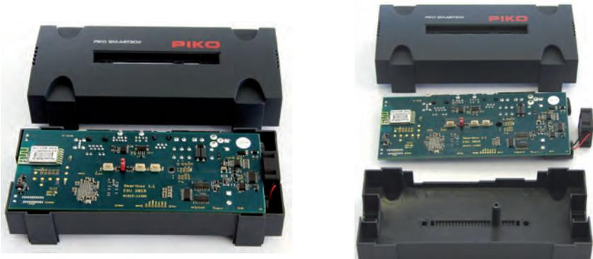
**Attention!** To avoid any possibility of short circuits cover the screw heads with electrical tape.
