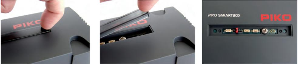
Next carefully remove the mainboard of the PIKO SmartBox® by lifting it up. The best way to do that is to use the two handling areas on the left and right side.
