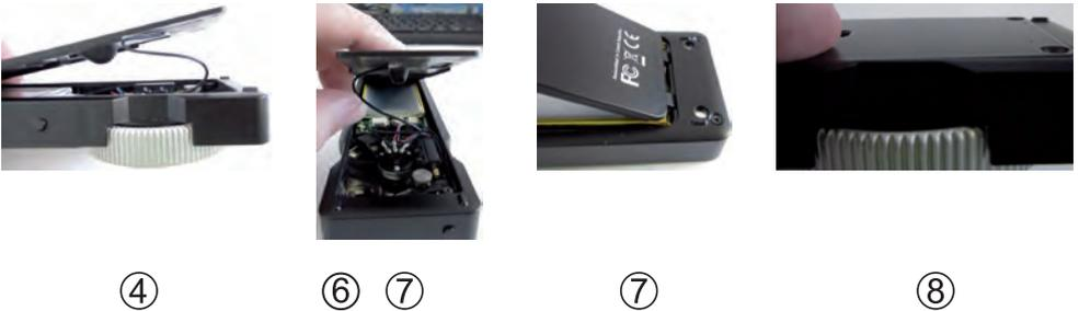
\*In case the wire attached to the cover is accidentally removed from the main circuit board. It can be easily plugged into the main circuit board again. The plug can be inserted either direction. For easier assembly we suggest placing the wire towards the front of the unit.
