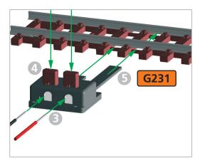
The mains plug (mains adapter) ① is connected via the small plug ② to the socket in the PIKO Digi 1. The two connection leads marked "A" on the bottom of the PIKO Digi 1 are first fixed in the connecting clip ③ by pressing the knobs ④ and are then connected to the rails as follows:
