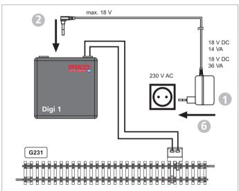
Please note: if you are using the PIKO Connecting Clip #55270 then the condenser in the clip MUST be removed. If the condenser is left in the Connecting Clip it will eliminate the high frequency control impulses and neither locos or accessories will work.
