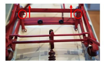
Now the scissor pantograph has no tractive forces of its own and is moved exclusively by the servo.
