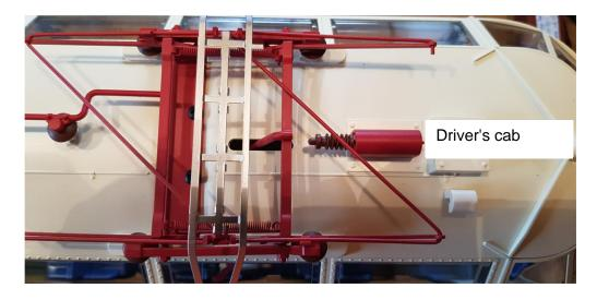
Extend the pantograph so that the springs have as little tension as possible. Unhook the springs on the driver's cab side first with tweezers. Then also on the other side.
