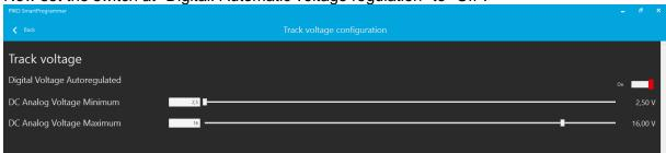
Now set the "Digital Voltage Maximum" to 10.5V - 11V by entering a number or using the slider.
