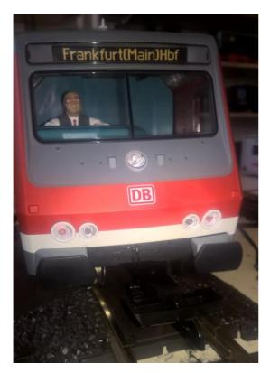
When F3 is turned on, the full beam of the control car is turned on.
