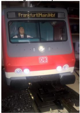
When F4 is turned on, the driving direction indicator of the control car is flashing.
