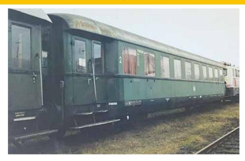
At the beginning of the 1930s, the DRG began building four-axle express train coaches to replace the older state railway designs with their three-axle running gear with more comfortable designs. Thus, over a period of about 15 years, various types of express train coaches were developed, culminating in the coaches of the type 42.
