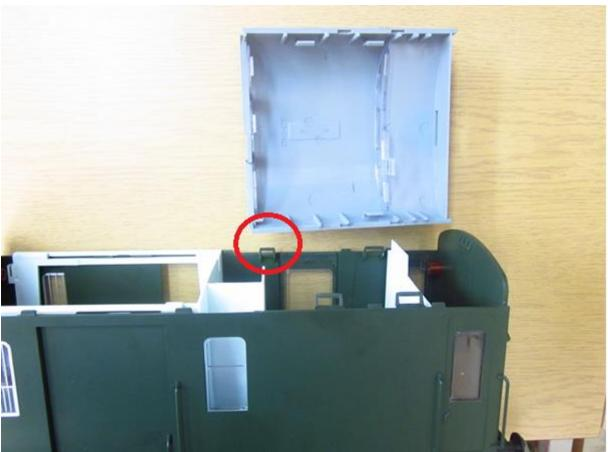
Release the latch and pull the pulpit roof upward with some force to release the remaining latches.
