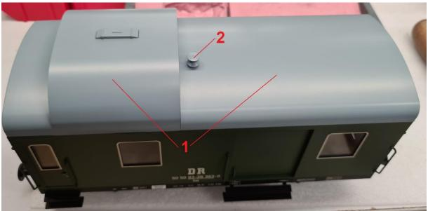
1) First, the roof is connected to the pre-assembled pulpit roof and mounted evenly on the car body.
