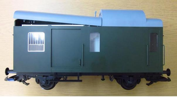
Pull the roof slightly forward and then remove it upward.
