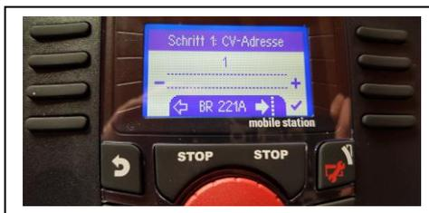
After a short display "Reading CV-value" the result will be shown immediately. In the factory setting of the locomotive decoder this is always address 3.
