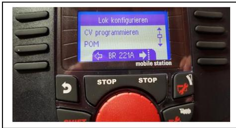
After this selection the DCC CV programming menu with the CV1 (locomotive address) appears directly.
