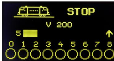
The display clearly shows all the information about the locomotive, the speed, the driving direction and the state of the locomotive's special functions or of the currently chosen operating mode (e. g. position of the switches in the **turnout mode**).
